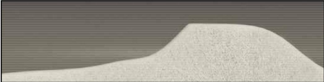
These illustrations provide a clear graphic representation of actual flow loop tests conducted at Stim-Lab. Above, uncoated Northern White frac sand shows behavior that's typical in traditional slickwater fracs. It drops out of the frac fluid and creates a duning effect that prevents proppant transport deep into the fracture.
