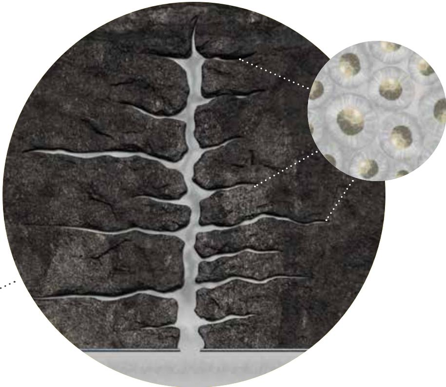
Our proprietary polymer coating swells to provide efficient thin fluid proppant transport deep into fracture tips. Propping open the fracture uniformly from wellbore to tip maximizes contact surface area for improved production.
