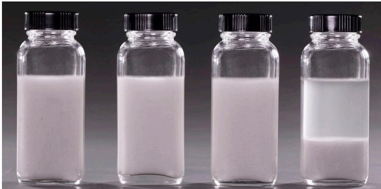
Propel SSP 350 in Fresh Water Propel SSP 350 in Brackish Water Propel SSP 350 in Produced Water Raw Sand in Slickwater
